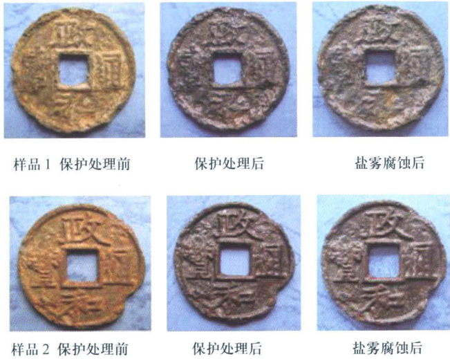
图 8 宋代铁钱在保护处理前、保护处理和盐雾腐蚀后的对比照片 Fig.8 The pictures showing the iron coins before and after conservation,after corruption test
