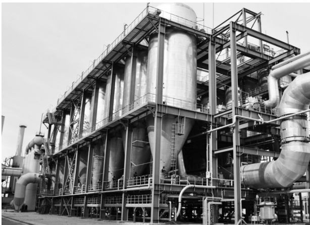
图5 迁钢高炉煤气干法除尘工程实景 Fig.5 Gas Dry-type Dedusting Field
